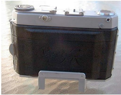
One other interesting feature of the Certo Six is the two folding legs on the back. These “legs” allow the camera to sit flat when the front is opened.
